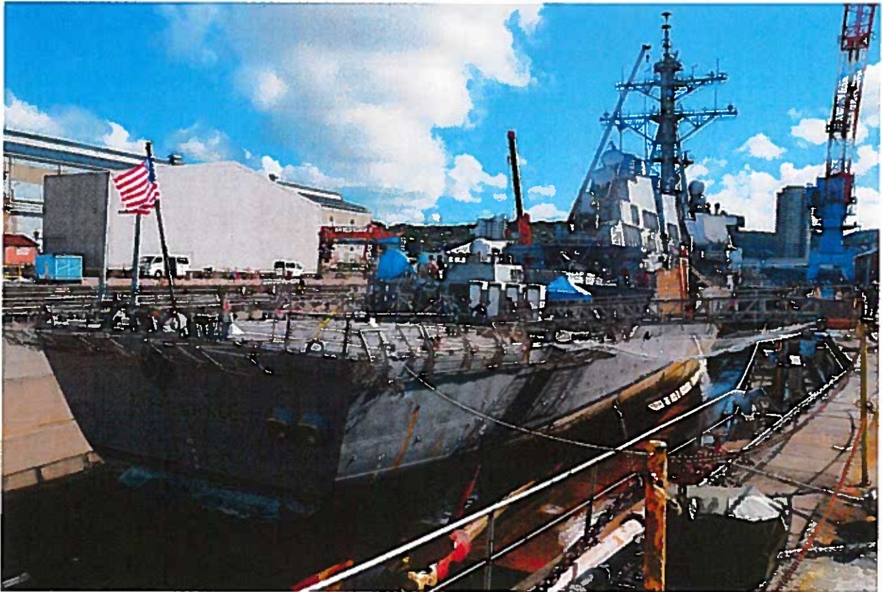
The USS Fitzgerald in a Navy repair yard after its collision with a merchant vessel off Japan in 2017 (Photo: U.S. Navy)
